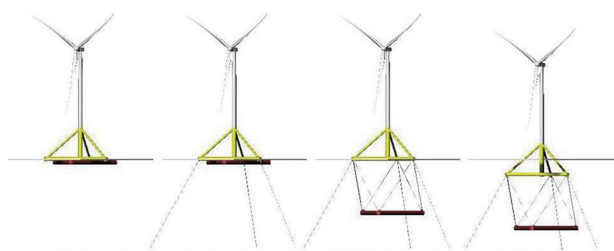
图8 TetraSpar 运输和安装过程中结构型式转变 [33] Fig. 8 Transition of TetraSpar during transportation and installation [33]
